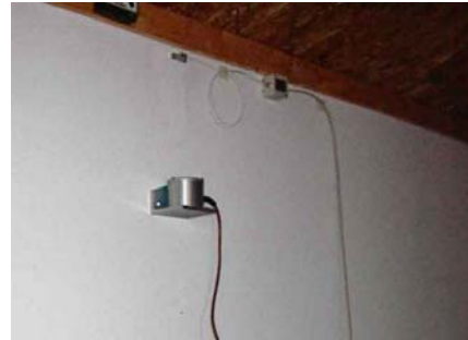
Tri-axial velocity geophone mounted below Kaman gage
