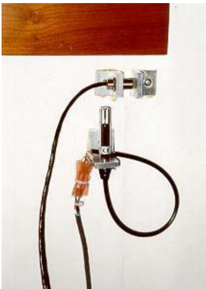
Kaman gage mounted over vertical crack (above), temperature/humidity sensor (below)
