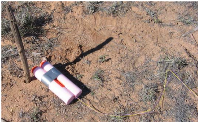
Fig. 1 Kinestik explosive charges
