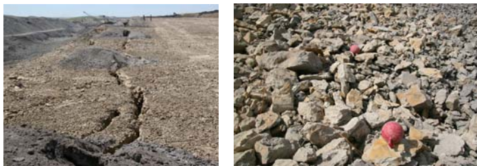
Fig. 2 Backbreak (left) and muckpile fragmentation (right)
