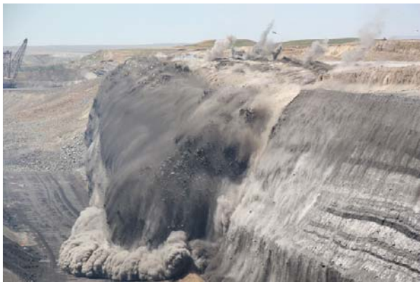
Fig. 1 Typical cast blast shot.
